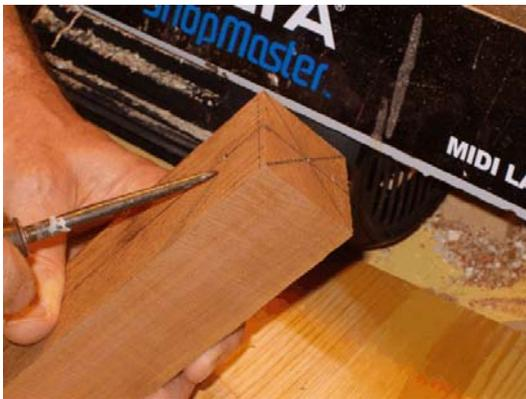
Before turning the body, I mark and drill the openings. It's easier to cut the openings before you turn the bodies shape.
