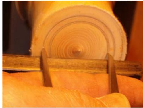
The cap (like the body) can be turned from scrap material. The cap material needs to be about 2in. in diameter and 3in. long. Once the cap material has been turned to a cylinder and the end has been squared, a divide can be used to find center. Notice, if the divide draws two circles, move the points until only one is drawn.
