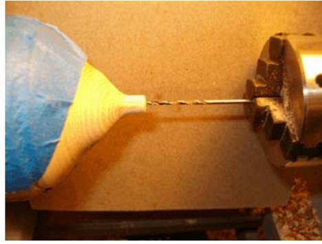
Once the cap is parted off, the stem can be drilled for the eyelet
