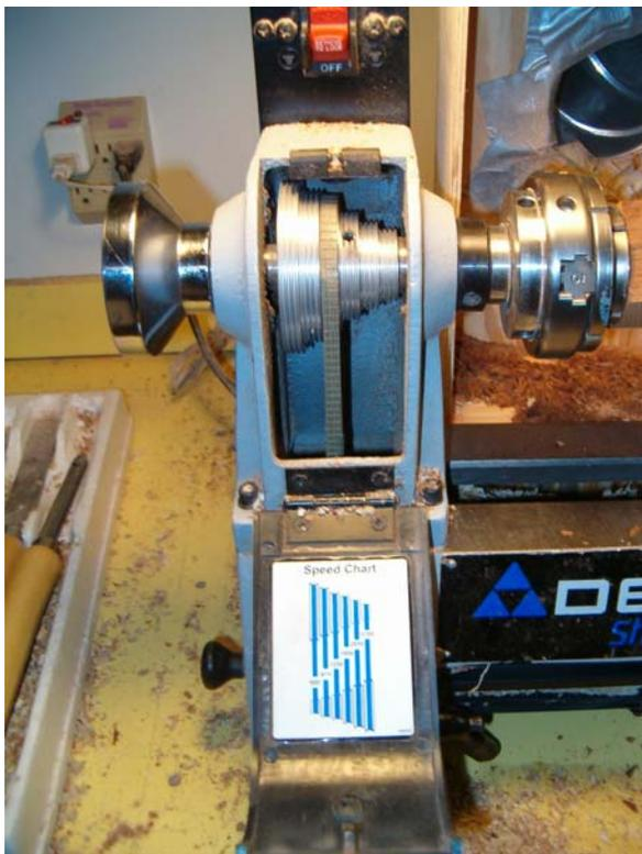
Don't forget to change the speed. I normally set the speed to, around 1200 RPM.
