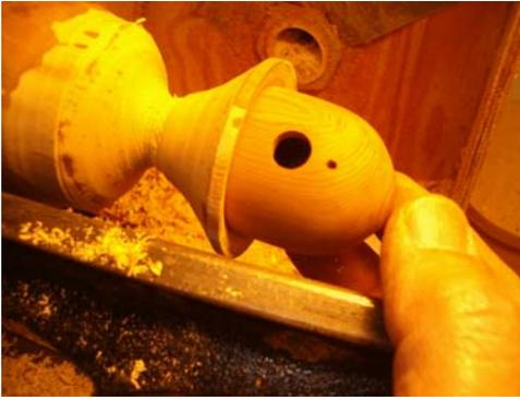
The cap can be used as a jam chuck to refine and sand the shape of the acorn body.
