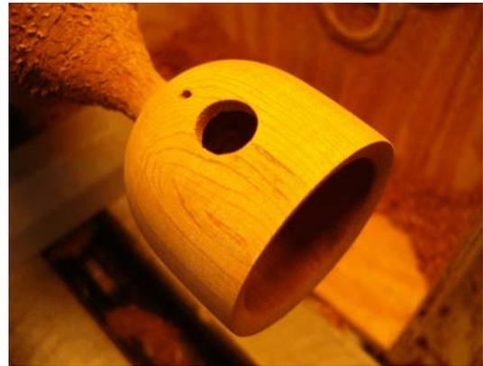
As you shape the body be careful not to remove too much material from the base. Before parting off the body it's a good idea to rough sand the body.
