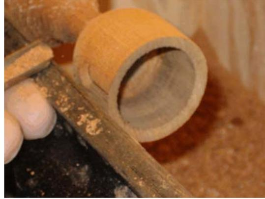
Now that all of the openings are cut in the body, use a roughing gouge to turn it to a cylinder. I shape the birdhouse using a 3/8 spindle gouge.
