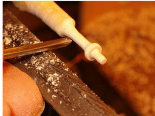
Now for the perch. With the material held in a three-jaw chuck use a small gouge to turn the perch to about 1/16in. diameter.
