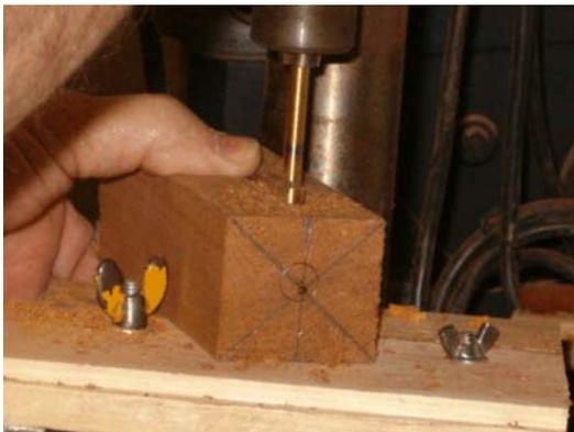
I drill a 3/8in. hole about a 1/2 to 3/4in. deep for the entry to the birdhouse and a 7/64in. hole for the perch.
