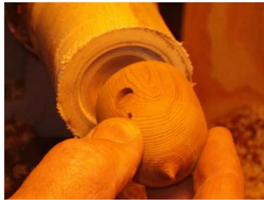
Once center has been established a cutoff tool can be used to fit the body and cap.
