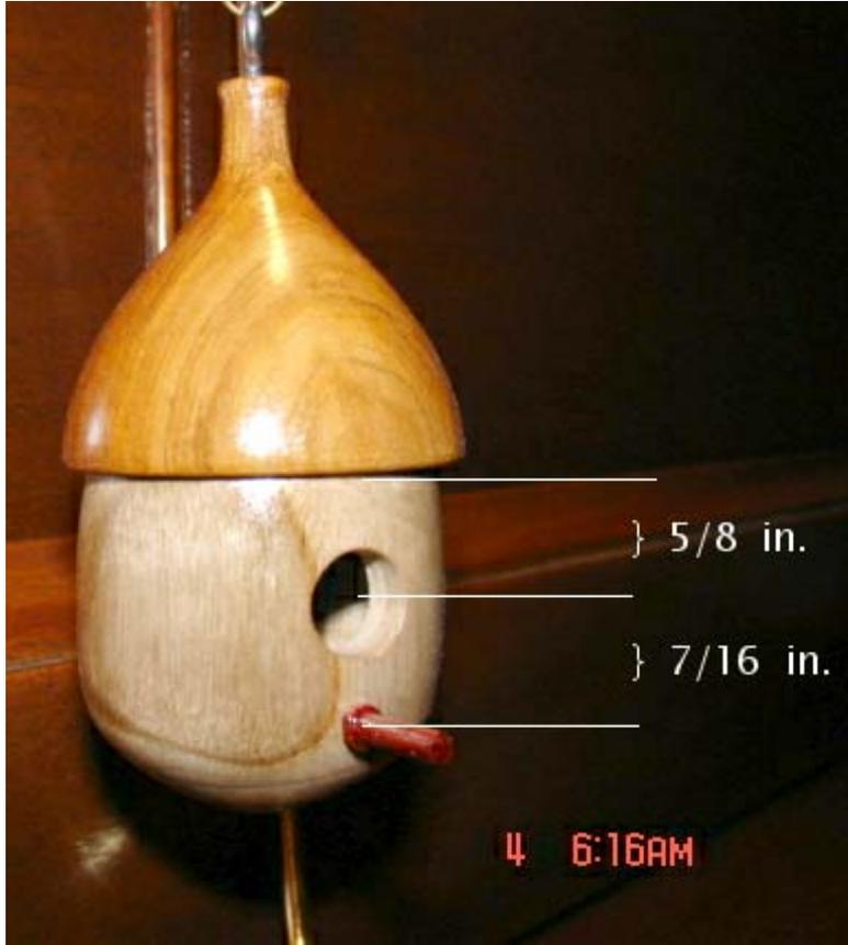
The body of the Acorn is made with square straight grained stock about 3in. long and about 1 1/4in. square.
