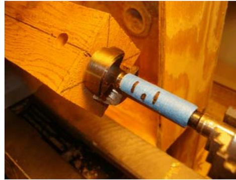
I use a forstner bit to hollow the body of the acorn. But, before I start hollowing, I slow the lathe to its slowest speed, about 500 RPM. The depth of the hollowing depends on the body design, but is usually between 1 to 1 ¼ inches.
