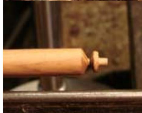
With the rest of the blank, make the clapper. Estimate the length you will need based on the distance from the top of the inside of the bell to the bottom.
