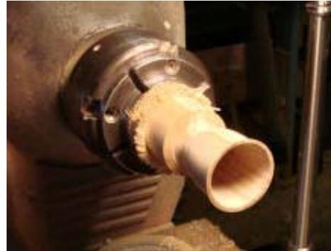
Drill a 5/32" hole in the inside of the bell at the top. This will be the mortise for the clapper tenon.
