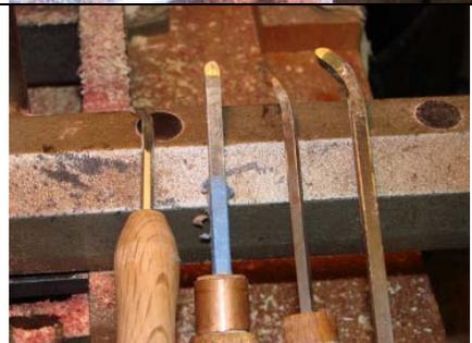
Simple tool made from a coat hanger to determine wall thickness. Direct from Dick Sing's books.
