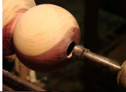
Use a flat scraper to create a flat seat for the cap
