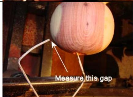
You now complete the exterior of the globe. You need to do this to check the wall thickness at the bottom of the globe.
