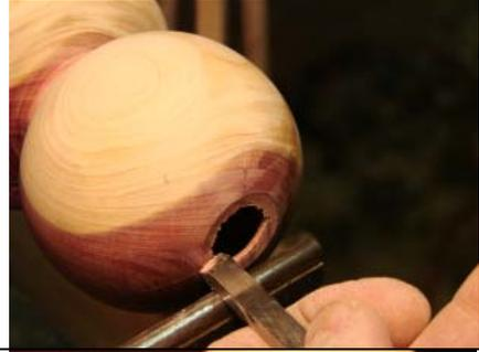
Use a parting tool to cut off the globe, as well as leaving a flat for the finial.
