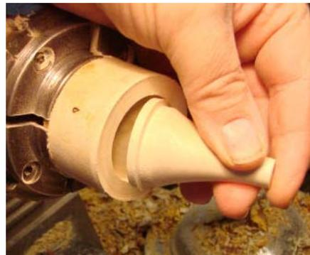
The depression is added with either a small gouge or skew.
