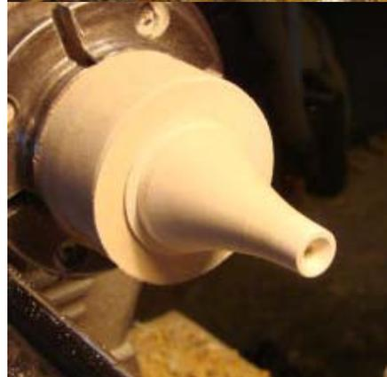
Add a bead of CA glue around the ledge in the body and insert the funnel.
