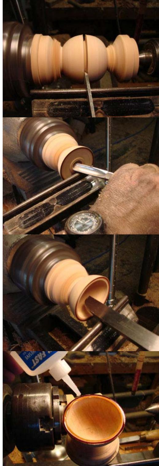
Clamp on lathe until the glue sets. Then begin to refine the outside. Take down the stock on each end to get close to where you want to part off.
