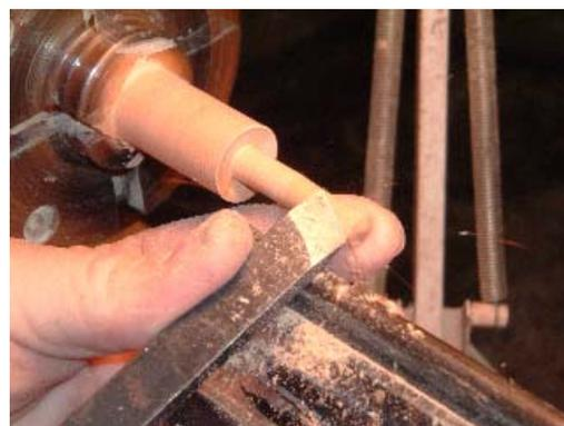
a skew or gouge to turn the upper section, shaping it nicely.
