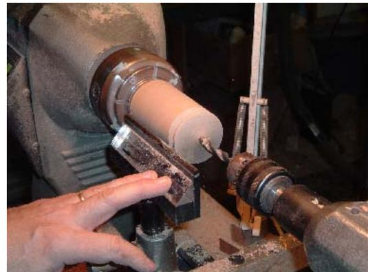
3. Start cutting the bottom of the top by cutting some relief area and then paring down with the skew. You can also use a parting tool to develop enough clearance, but remember there is a 5/16" hole drilled so don't go too deep. Finish forming the disk and part off the disk with the skew.
