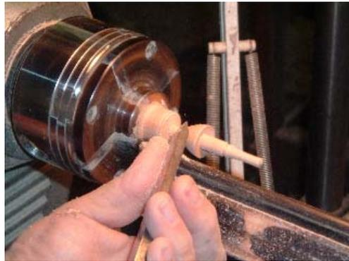
8. Finish the disk separately if you want to paint or marble the disk. Use CA glue to join to the stem and then apply finish to the completed top.
