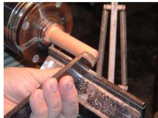
6. The stem has three sections. The top part is where you spin the top from. The second part is a  $5/16$ " cylindrical section that fits tightly through the disk and the bottom section is the bottom of the top tapered to a fine point. Use a parting tool to establish the bottom of the second section and then use
