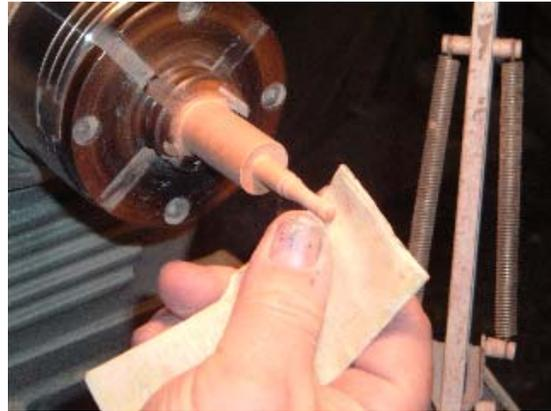
7. Form the bottom section. This should be the full 3/4" diameter and gently slope to a sharp point. This section shouldn't be too long, between 1/2" and 5/8", otherwise the top could be top-heavy. Take it very easy at the point and don't push too hard since you don't want to brake off the point. You need to cut as sharp a point as possible to maximize how well the top spins.
