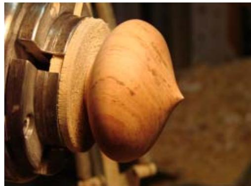
Start the stem by turning a 5/8" tenon and then begin to refine the transition to the base of the stem.
