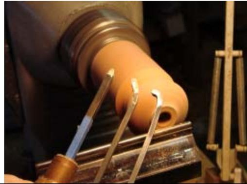
Use a gauge to measure the wall thickness. Walls should be about 1/8" thick on the top half.
