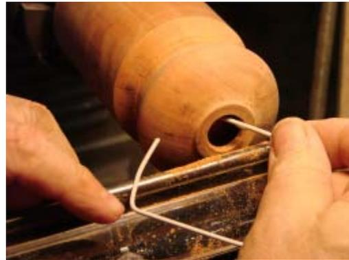
Refine the bottom of the top making a nice reverse curve to a sharp point. Part off with a sharp gouge or a skew.
