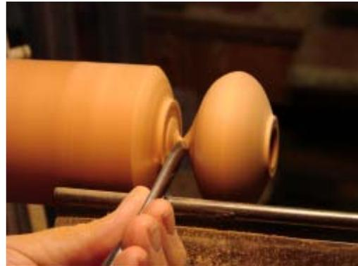
Make a jamb chuck with a 5/8" tenon. Mount the top and refine the point with a skew if required and then finish sanding.
