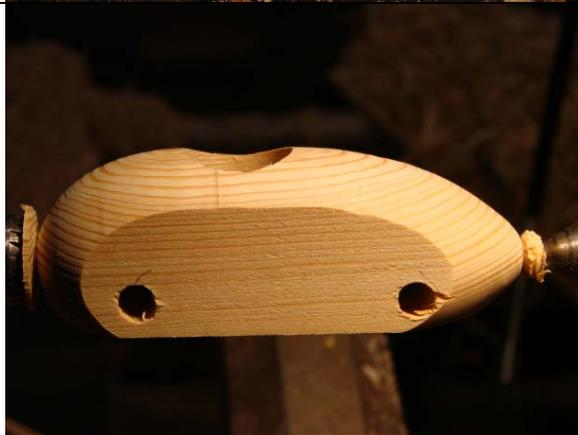
Remove the car from the lathe and cut off the buttons on the end. Sand the nose and tail smooth.
