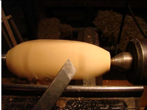
Turn the ends until you are almost cut through at each end. You can sand the nose and tail a bit while the lathe is on, but be careful. Sand the top smooth of any tool marks by sanding with the grain and the lathe off.
