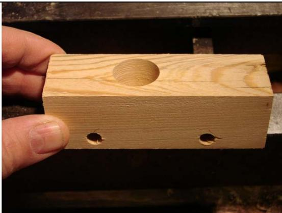
Mark the ends for the offset, about  $\frac{3}{8}$ " toward the bottom of the car, ie. the axel hole side. Repeat on both sides
