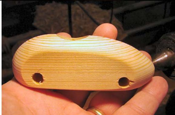
Cut axels to give about 1/8" play, so the wheels turn freely. Note the two different hole diameters in these 1" wheels.
