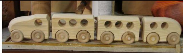
In this case I cut the blanks 1 1/2" wide, by 2 1/4" tall and 4" long. I used 1 1/4" wheels here and drilled a 1 3/8" counterbore to recess the wheels. I did this by first drilling the counterbore on one side, then through drilling with an 1/8" bit through the center of the counterbore to locate the center on the other side, After the counterbores, I drilled for the axels. Drill the windows with a 3/4" bit.
