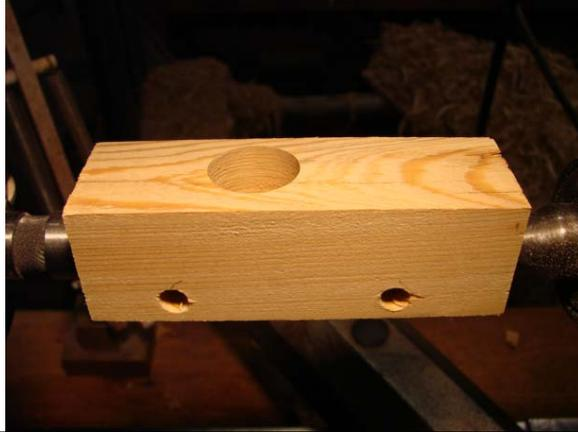
Use a skew or a spindle gouge to round over the top and form the ends. You just want to remove the flat from the top. Make sure you don't cut too much around the wheel area, since the wheel needs some flat area to keep the wheels free turning.
