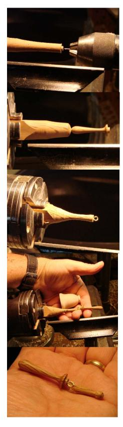
Add a little CA on the top of the button on the bell and then slip the clapper through the ½" hole and you're done.
