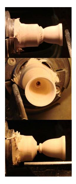
Chuck up a blank for the handle and clapper. This should be a fine grain wood. I usually start with a ¾" square blank. Turn the handle with a ¼" tenon on the bottom. Check the fit with the bell.
