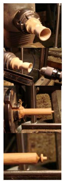
With the rest of the blank, make the clapper. Estimate the length you will need based on the distance from the top of the inside of the bell to the bottom.
