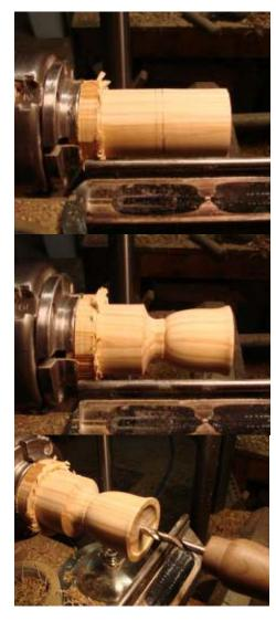
Hollow the bell using your favorite hollowing tool. Get the bell fairly thin, 1/8" or less, to reduce the weight of the ornament. Shear scrape the inside to the final wall thickness, then sand both the inside and outside of the bell.
