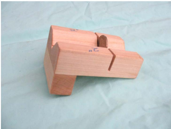
Two self explanatory views. Choose a stop material which will be stable to repeated sharp gouges and yet will not nick the sharp gouges. Copper, brass, hard plastic or a quarter can be used. Glue in place (epoxy was used in this jig).
