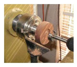
Using the 1 3/8 bit, I drill another hole on the face of the piece. Now I have two holes centered on the piece so I can flip the piece from front to back and maintain centering.
