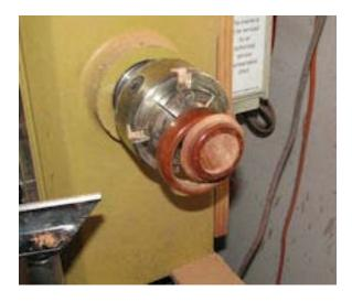
Here's where I kind of departed from what I saw in the various articles and made my own version of a "chuck" to hold the piece so I could finish off the inside.
