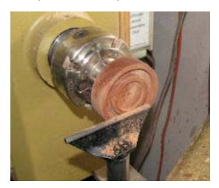
Using a parting tool begin to form the shape of the bangle at the piece where you made the mark. You can flip the piece from front to back and back to front a few times to get things even. Don't part too far; you want to sand and finish the piece at this point.
