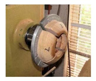
Using my mini-cole jaws, I attached a ring of 1 1/2 inch stock and turned a recess to hold the bangle. The recess was smaller than the bangle would be. I took the ring off the cole jaws and quartered it on the band saw.
