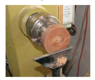
Now I mark a 2 3/8 to 2 1/2 inch circle on the face of the piece with a compass. I do this with the lath off. Place the point of the compass in the dimple made by the drill bit and rotate the piece by hand.
