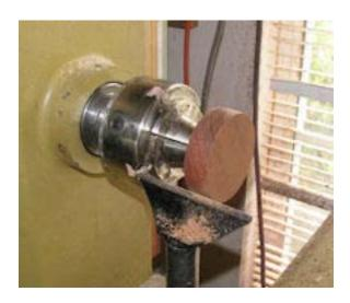
True up the diameter of the blank. Since I use dimensioned lumber for my bangles, I don't worry about truing up the face. Most of it will disappear eventually anyway. Since this is a face grain piece, I use a bowl gouge.
