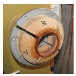
You now have access to the inside of the piece and you can flip the piece any number of times to finish the inside.
