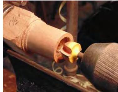
Forn the shape of the cap, including a small stem. Part off, leaving a nice stem.
