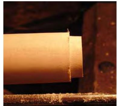
Refine the cap, doing the final shaping on the stem and top of the cap and sand. Then begin the texturing process with the Wagner Texturing Tool.
