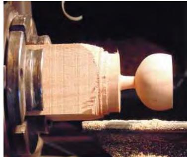
Next, mount a lighter colored wood in the chuck. This blank is maple, about 1" thick and turn to a cylinder.
