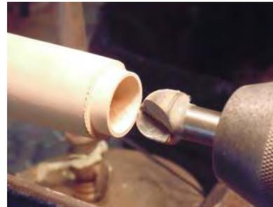
Roughly turn the nut shape and part off. Create another jamb chuck for the nut to fit on and refine the shape and sand.
