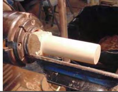
Rather than turn the nut right away, we're first going to turn the blank into a jamb chuck to finish the cap. Measure the inside of the cap with pair of calipers.
