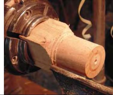
Use a Forstner bit, mounted in a Jacob's chuck to drill a hole about 1/4 - 5/16" deep. The deeper the hole, the less likely that the nut will slip off the cap. For a 1 1/2" wide cap, use a 7/8" drill
