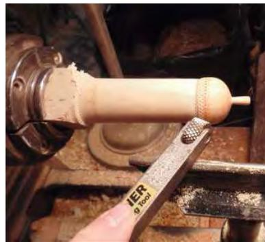
After the first band of texturing, pull back the tool and move it up to the next band. Lightly press the tool to the wood and let it reengage in the previous pattern, then press hard. Repeat up to the stem.
