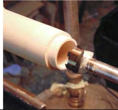
Just as in the cap, round the bottom of the nut, either with a scraper or a  $\frac{3}{4}$ " box core router bit.
