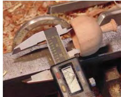
Turn a tenon on the end of the blank to just larger than the calipers. Put a slight taper on it and keep on refining the tenon until you get a tight fit with the cap.
