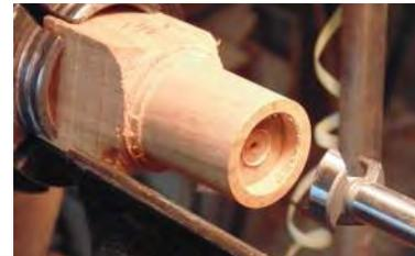
To make the underside of the cap rounded, you can either use a round nose scraper, or use a 7/8" core box router bit, mounted in the Jacob's chuck.
