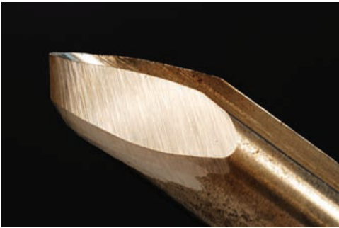
This 3/8" bowl gouge has a fingernail grind.
