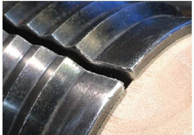
2mm gap between adjacent jaws to allow for the kerf of the saw blade that was used to cut them into four jaws. When cutting a recess in a bowl blank for the outside of dovetail jaws to expand into, make the recess just larger than the jaws
