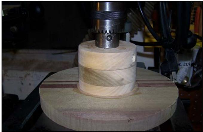
**Figure 8:** I use my drill press to apply clamping pressure at this step. Center the waste block and bowl blank on your drill press table, and raise the table until it presses up against the drill chuck.
