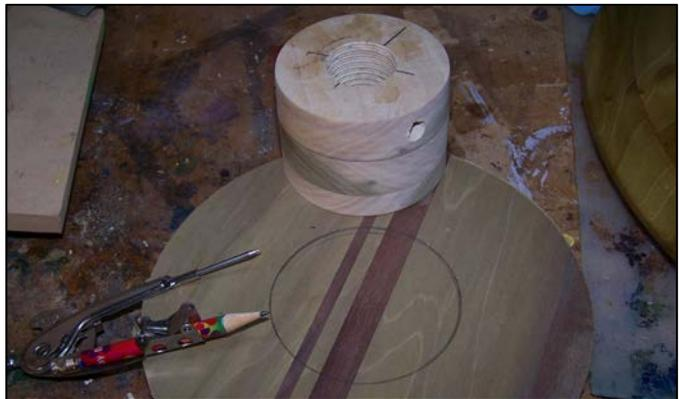
**Figure 7:** Mark the center of the blank with a compass just slightly larger than your waste block. This will help align the block when you glue it to your bowl blank
