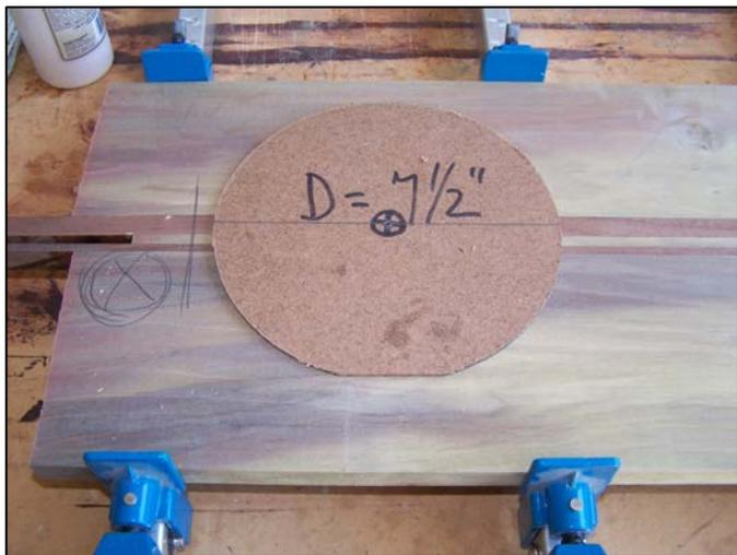
**Figure 3:** Plane the boards flat on both faces, and use a template to lay out your bowl blank in the correct diameter.
