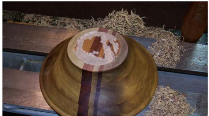
**Figure 15:** *Break apart your paper bag glue-up with a mallet and sharp chisel. You get a nice clean break with only some paper residue (no split wood or screw holes) that's very easy to sand or turn away.*
