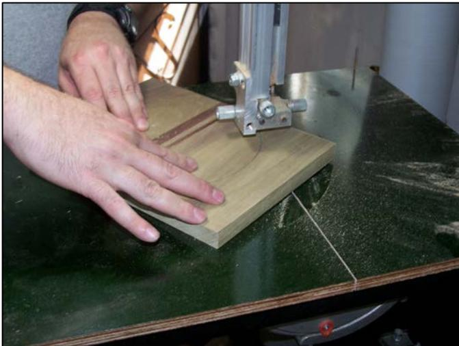
**Figure 5:** A circle-cutting jig makes it easy to cut the blanks round. But you can free-hand it if you are comfortable with that.
