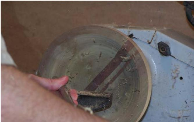
**Figure 14:** *Turn the inside of the bowl first, being careful to only remove enough wood to even out the rings.*
