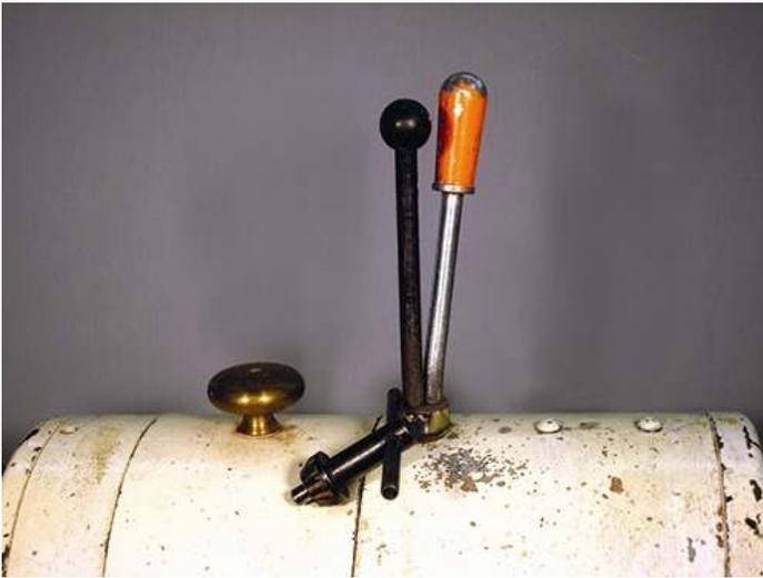
Are you always searching for the chuck key or toggle bar? Do you have to stoop or turn around to pick it up every time you need it? Wouldn't it be nice if it were always right on top of the headstock, inches from where you are going to use it? Help is at hand. Epoxy a rare-earth magnet to the top of the headstock and you are done. One magnet will hold several items at a time.
