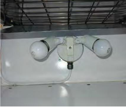
**The lightbulbs are mounted on the back of the kiln near the bottom, a sheet of metal covers the bulbs, and the holes are drilled through the bottom of the freezer.**
